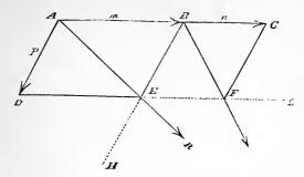
Let A be the particle on which the forces act. Draw AB, AD representing the forces m and p respectively in magnitude and direction.
